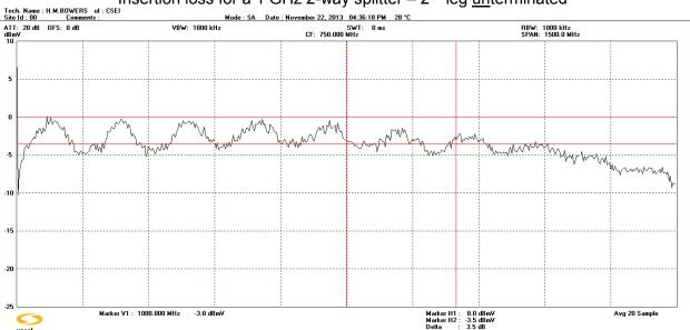
Insertion loss for a 1 GHz 2-way splitter – 2<sup>nd</sup> leg unterminated
