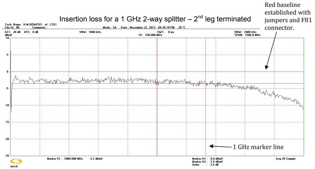
The red line at 0 dBmV marks the baseline (jumper from noise generator to analyzer input using short cables and a F81 connector) response of the noise generator out to 1.5 GHz and beyond. The black line represents the throughput loss from splitter input through one of the two output legs, with the other output properly terminated. Loss at 1 GHz is approx. 3.5 dB! The loss at 1.5 GHz, however, is >10 dB!
