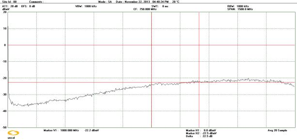
'Tap port' to 'Thru port' Isolation for a 1 GHz DC-12 coupler – Coupler Input Terminated
