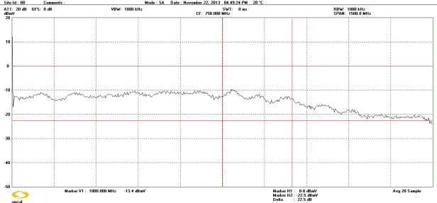
'Tap port' to 'Thru port ' Isolation for a 1 GHz DC-12 coupler – Coupler Input <u>Un</u>terminated
