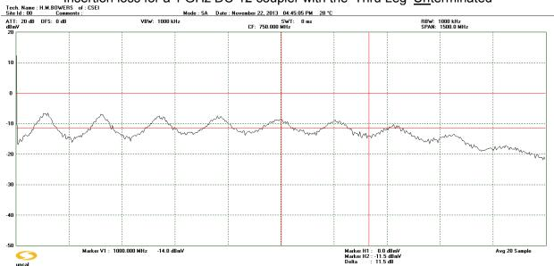
Insertion loss for a 1 GHz DC-12 coupler with the 'Thru Leg' Unterminated
