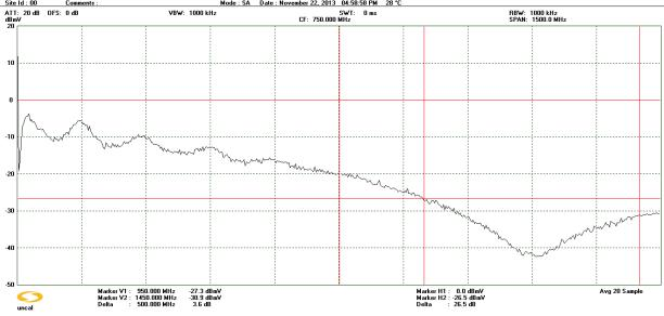
4W L-Band Splitter – Isolation Between Two Output ports with Other Legs Properly Terminated.
