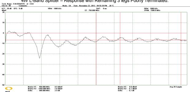
4W L-Band Splitter – Response with Remaining 3 legs Poorly Terminated.
