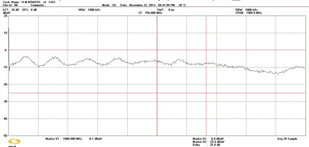
Port to port isolation for a 1 GHz 2-way splitter – 2W input is unterminated
