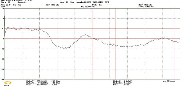
4W L-Band Splitter – Isolation Between Two Output ports with Other Legs Poorly Terminated.
