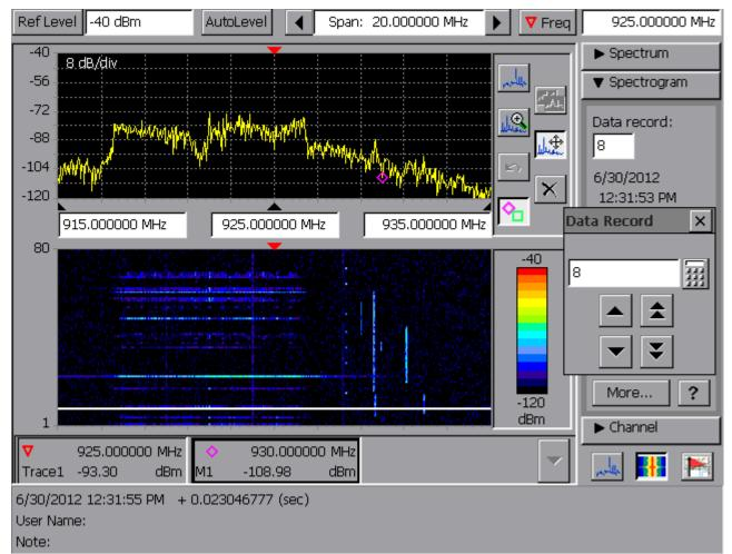
In the 1st Quarter 2012 Technical Report we examined some very active spectrum from 915 to 935 MHz. Selecting data record 8 in the spectrogram above, we can see considerable spectral activity. The spectrum from approx. 917 to 927 MHz 'appears' to be digital in nature (QAM, VSB, PSK, etc.), along with what appears to be many low level analog carriers in the 929 to 934 MHz region.
