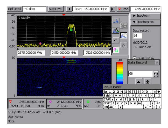
Advancing the spectrogram to data record 68 shows a transmission from the nearby router on WIFI Ch11. The point of these past two screenshots is to demonstrate how the spectrogram enables capturing and later analysis of intermittent signals. Spectrograms can be recorded to disk (hard or thumb drive) to monitor spectrum, if necessary, for long periods of time. Recordings can be continuous; or be set to trigger and record by time interval or when a 'limit line' is exceeded.
