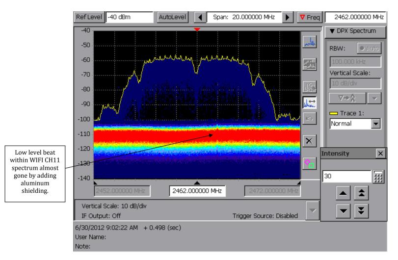
Note that the beat is now significantly reduced in amplitude through the addition of some aluminum shielding between the antenna and interferring source direction.
