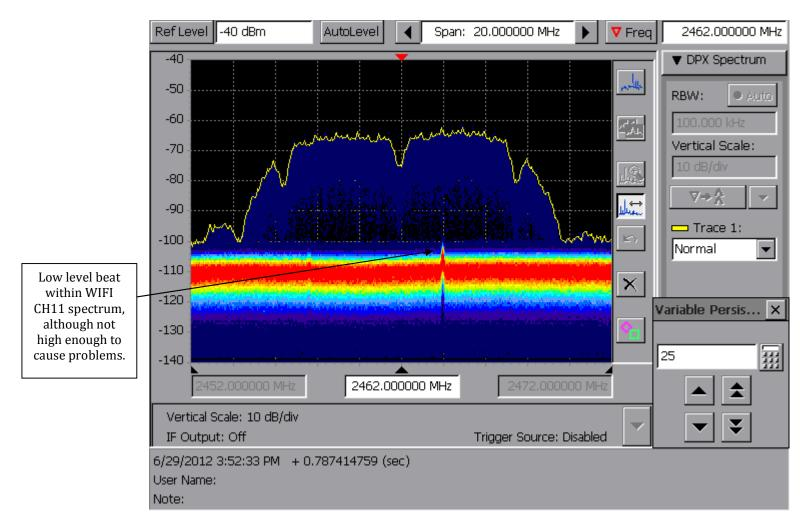
I've now switched to WIFI CH11, the router physically closer to the analyzer. Although router spectrum and activity generally looks OK, note the low-level 'beat' within the spectrum. This carrier is from a distant source as shown in the next slide, and is not high enough in amplitude to cause packet loss problems; however it's still interesting to note it's presence and that it can be measured. See the next several slides for further illustration.
