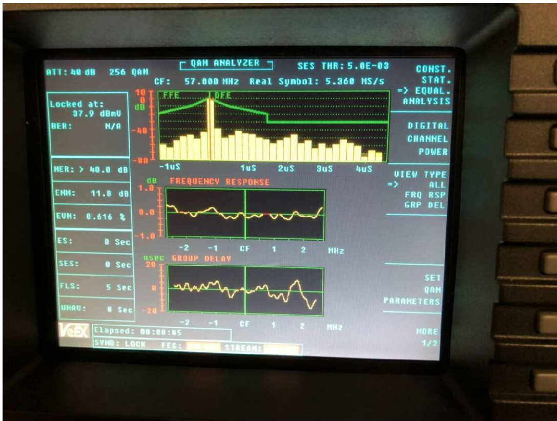
QAM measurements on Ch61 in lab. Many test results are shown including MER, ENM, EVM, adaptive EQ activity, frequency response & group delay.
