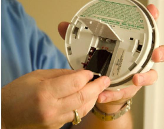
Smoke alarms are powered by battery or they are hardwired into the home's electrical system. If the smoke alarm is powered by battery, it runs on either a disposable 9-volt battery or a non-replaceable 10-year lithium ("long-life") battery. A backup battery is usually present on hardwired alarms and may need to be replaced.
