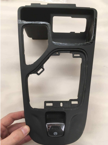
Picture 3 (Shows what to trim off the bottom side for fitment of the rocker switches and relocation of the media center / 12 volt socket)
