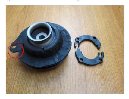
Since the strut top mount will be mounted to the suspension assembly for installation, we recommend mocking up fitment to vehicle with the factory strut top mount settings in place. (Align the hole with the plastic protrusion) located on the body of the vehicle where the strut mounts to. Now remove the strut from the vehicle, and hold the shock assembly and carefully rotate the strut top hat 180 degree clockwise. If you are having some resistance, carefully loosen the top mount nut 1-2 turns.
