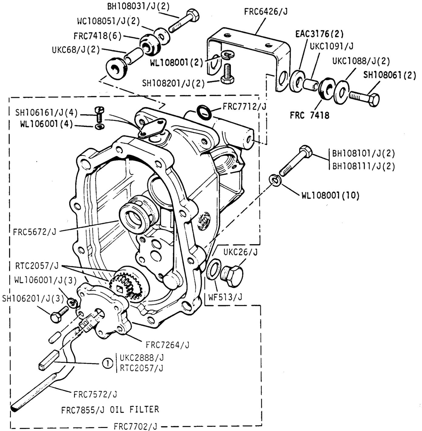
① RTC2057 - Gear Kit Oil Pump
