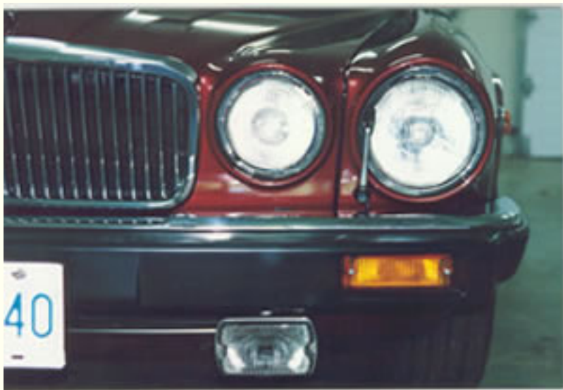
Original configuration H4 outer lamps, with Cibie driving lamps
