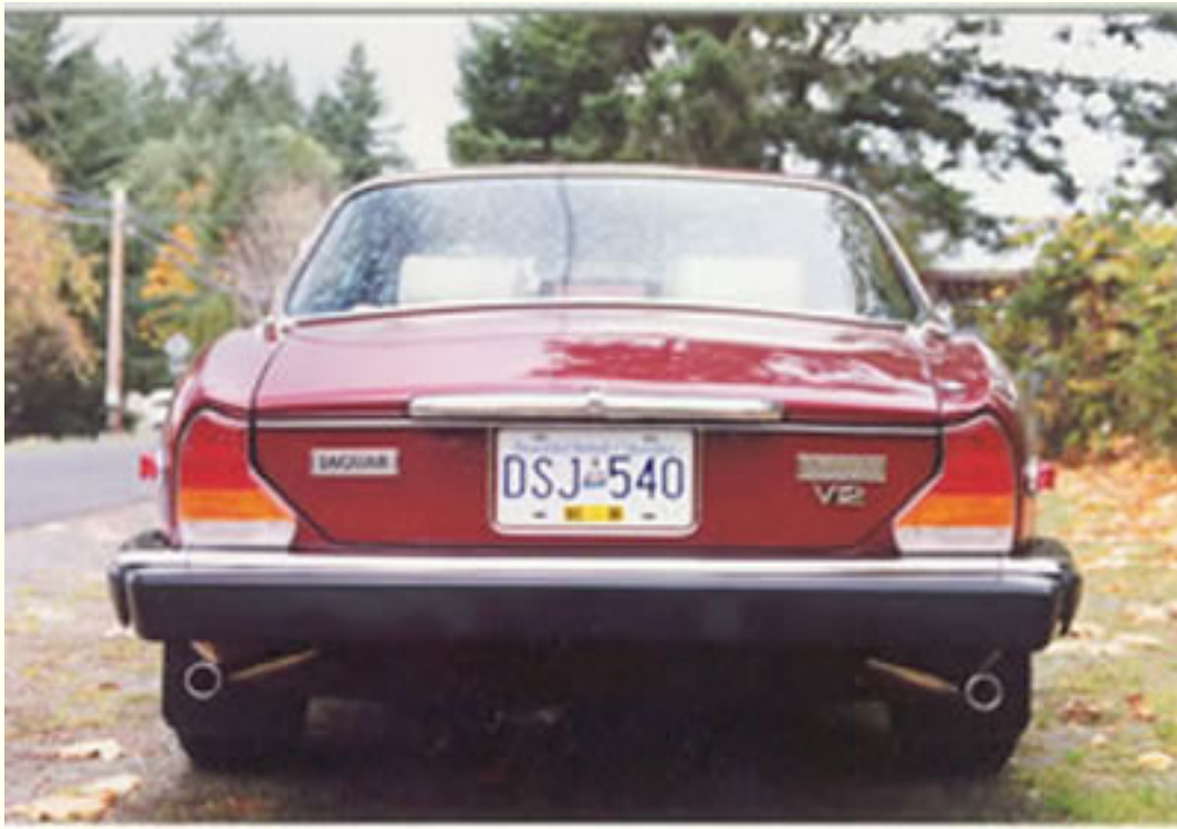
Correct placement of North American exhaust finishers
