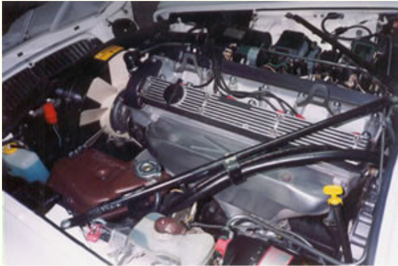
6 Cylinder Engine - Note white cooling fan.
