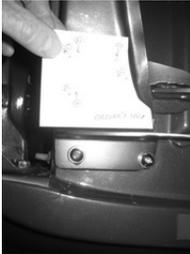
Center punch all 3 marks. Remove the template and drill the top two holes with a 5/16" bit. Install 2 new 5/16x3/4 bolts with nylock nut underneath.
