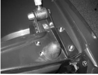
Install nuts onto rod ends. Screw rod ends into aluminum tubes, 1 RH & 1 LH threads. I recommend to use anti-seize on these parts. Screw these all the way in and then adjust the length to 16" center to center. When you turn the tube both ends will screw out for adjusting.
