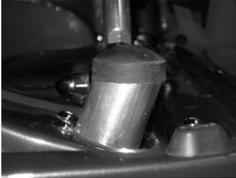
With the help from at least one person, preferably two, install the hood to the rod ends using the 1/2x5 bolts. Put one washer over the bolt, slide the bolt into the rod end, put a washer between the rod end and the hood bracket. Push the bolt all the way into the hood bracket and install the nylock nut.
