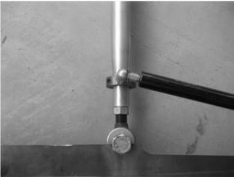
Parallel the tubes to approximately 63 1/2" apart center of rod end to center of rod end. Snug the bolts on the hinge bracket.
