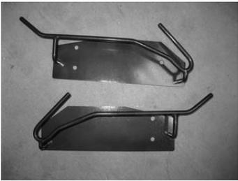
Remove the battery side mount that goes to the inner fender apron if it is still on the truck.
