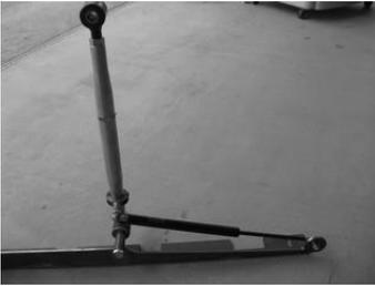
**This is important because the gas shocks will push on the jam nuts. If they are installed improperly, they will push on the tubes, loosen the jam nuts and pop the gas shocks out of the mounting balls.**
