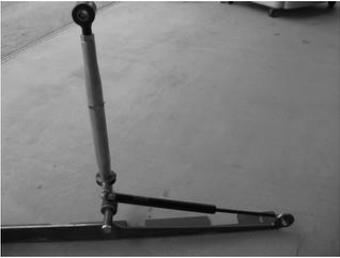
**This is important because the gas shocks will push on the jam nuts. If they are installed improperly, they will push on the tubes, loosen the jam nuts and pop the gas shocks out of the mounting balls.**
