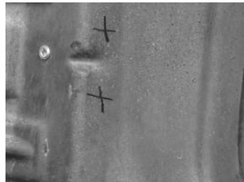
Be careful not to bind the hole saw and dimple the outside of the hood. Install the 3<sup>rd</sup> bolt(5/16") with a flat washer on the bolt along with a flat washer and nylock nut inside of the hood. Install supplied plastic plug after all bolts are tightened for the final time. Repeat for the opposite side.
