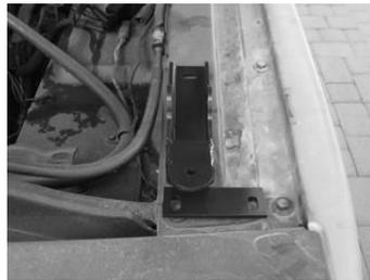
Install 2 new 5/16" X 1 ¼" bolts with flat washers. Mark the center of the rear slotted hole, remove the bracket and drill a 5/16 hole. Reinstall the hinge bracket with a 5/16" X 1 ¼" bolt with a flat washer on the bolt and a flat washer and nylock nut on the bottom. Leave these loose at this time. Repeat for the opposite side.
