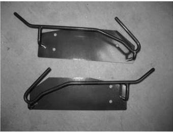
Remove the battery side mount that goes to the inner fender apron if it is still on the truck.
