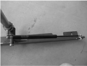
With an assistant, install the hood assembly back into the hinge bracket, re-install the bolts, nuts and tighten. Tighten all nuts and bolts at this time.
